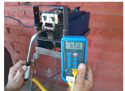
Pyrometer indicating proper blade temperature of 650°C.
