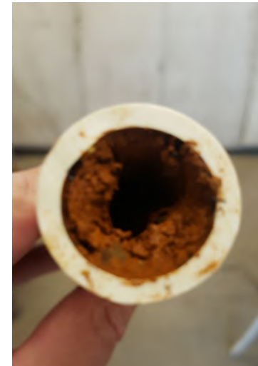
Biofilms and organic material can build up in water lines over time leading to reduced water flow.
