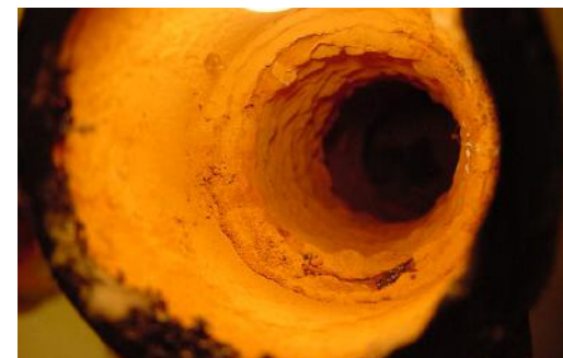
Biofilms and organic material can build up in water lines over time leading to reduced water flow.
