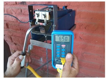
Pyrometer indicating proper blade temperature of 650°C.
