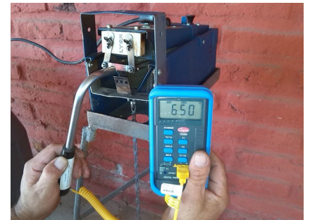
Pyrometer indicating proper blade temperature of 650°C.
