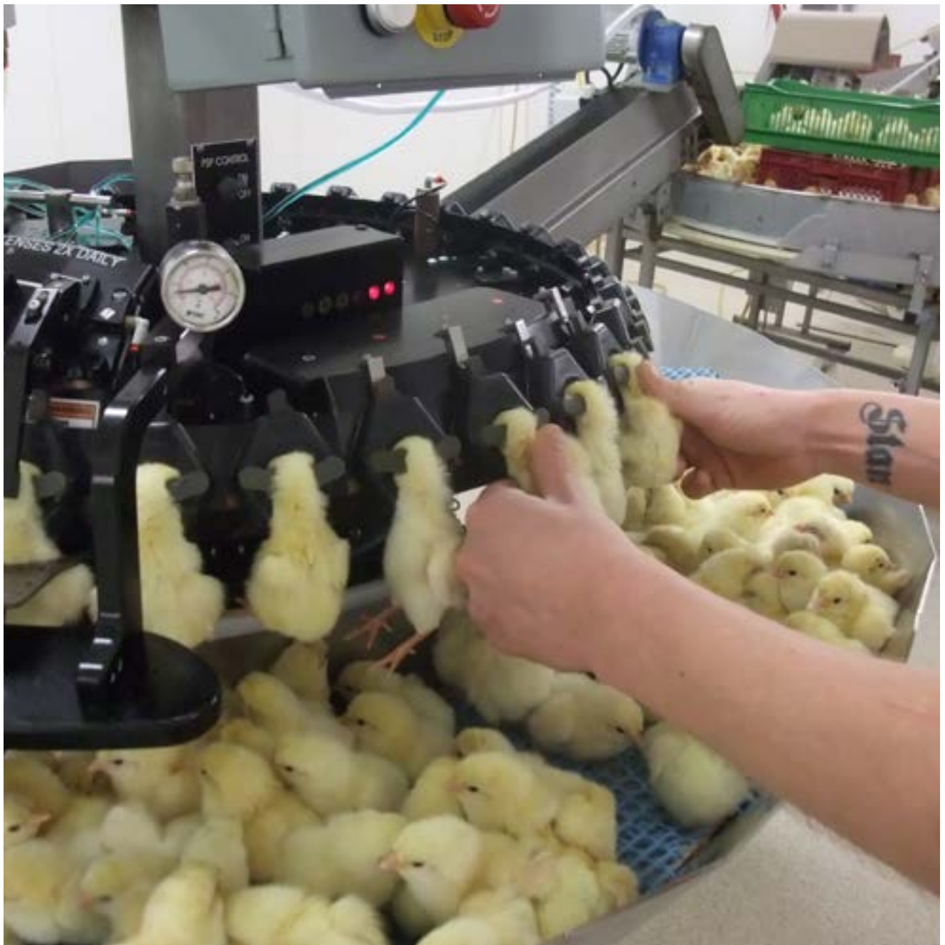
Latest innovations in hatchery equipment technology combine vaccination and infra-red beak trimming
