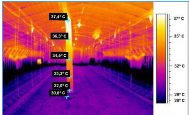
Temperature always has a height gradient. Careful consideration should be taken in cage systems. Courtesy of M. Czarick – UGA
